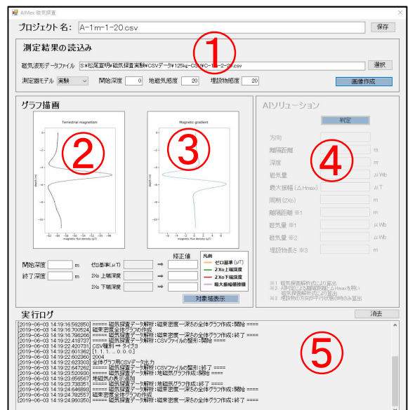
図-3 AlMex(AI magnetic exploration analysis)画面
